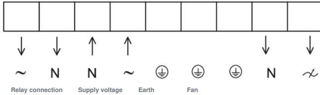
Transmission: between ~ and N is always 230V when the transformer handle is in pos. 1-5
