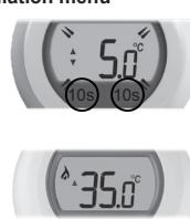
While this setting is flashing, touch the left touch zone briefly to display the minimum temperature limit. This can also be changed using the setting ring.
