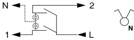
Two-circuit switch with indicator light
