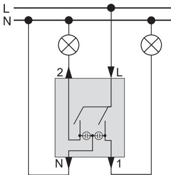
Two-circuit switch with indicator light
