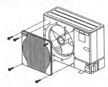
(3) Insert the stoppers (four locations) of the fan guard into the installation holes on the outdoor unit.
