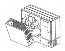
(2) Insert the fan guard stoppers into the square holes on the air guide.
